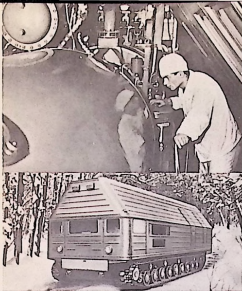
USSR now produces this small mobile atomic power station, which can travel almost anywhere, and supplies electricity in remote Arctic and desert regions, far from power.
