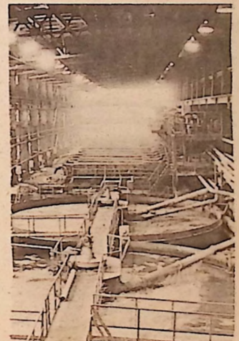
Potash rock here is very pure, but has to go through much processing. Here's a section of one concentrating plant where ground rock, made into a mud with water, is cleaned.
