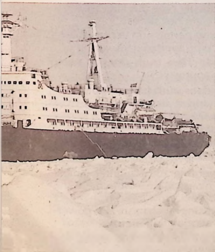
...rst nuclear-powered ice-breaker, has In that time of service with the Soviet owns. Indeed, it's nuclear power plant e have no figures on how much diesel the "Lenin" takes only "shovels" of fuel ired by standard breakers. Biggest nning out of fuel in the most terrible
