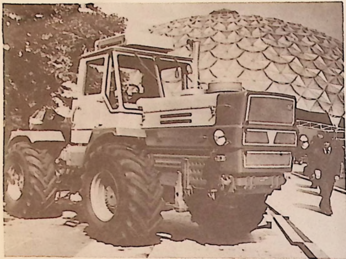
New T-150K is primarily for farming and, with attachments, can do all jobs on the land. Mainly for their huge Co-Op and State Farms. Powered by 165 HP turbo-charged diesel. Fully hinged under-carriage. Twelve forward speeds, four in reverse. Weight 8135 Kg (18,000 lbs). With speed of 30 KM per hour, can be used for transport. Selling abroad.
