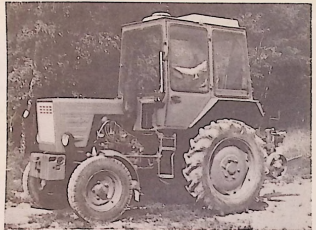
T-25A intended mainly for vegetable and fruit crops, and hay harvesting operates many attachments. New version of tractor popular in many countries now. Has 25 HP diesel, eight forward speeds, six reverse. Remarkably adjustable two ways: you can raise clearance from 435 to 642 mm, and increase width of tread from 1200 to 1480 mm. Speed up to 22 KM per house.
