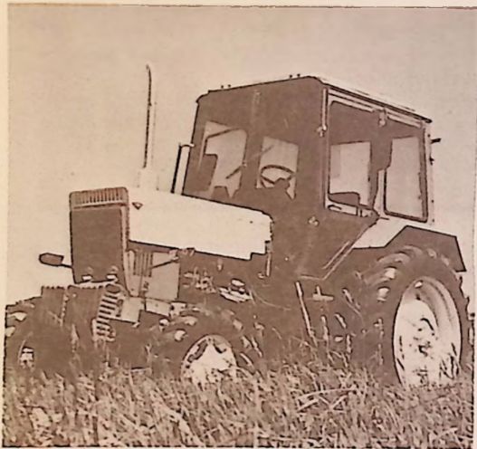
New 80 HP model of popular Belarus, the MTZ-82 has 33 KM per hour speed, with 22 forward gears. High clearance (640 mm) and both front and rear tread adjustable.
