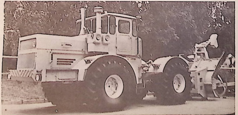
K-701 is for big farm and road jobs, with 275 HP diesel. Its main frame is hinged, for use with modern high-efficiency implements. Designed for new intensive farming methods being applied on tens of millions of acres. Unlike our machinery plants, in USSR they can't cope with demand, even working three shifts.
