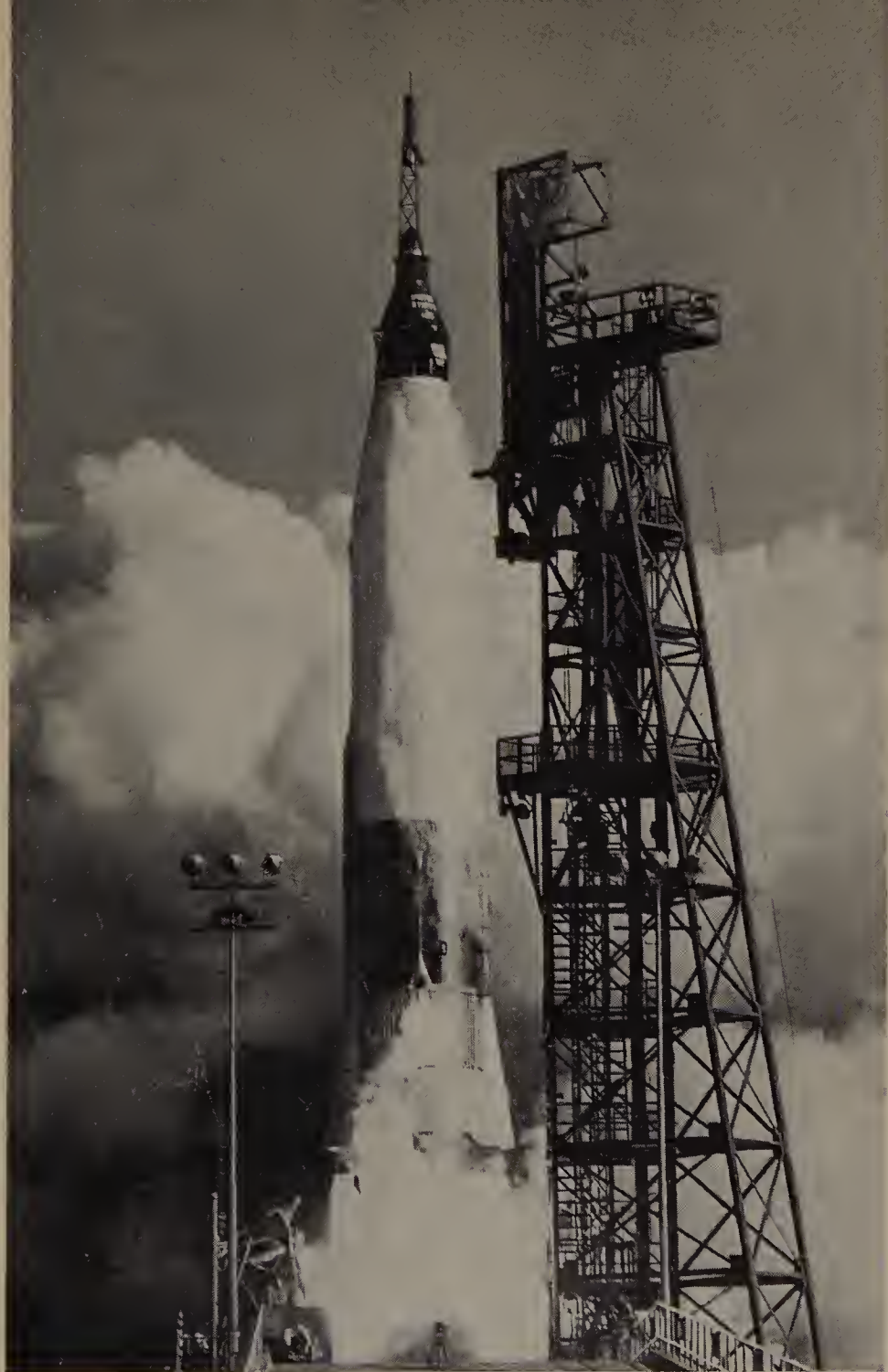
PLATE XLV AN Atlas ROCKET LAUNCHES THE SPACE-SHIP CARRYING JOHN GLENN. HIS CAPSULE IS THE CONICAL PORTION JUST BELOW THE TRELLIS GIRDERS AT THE TOP. (p. 284)
