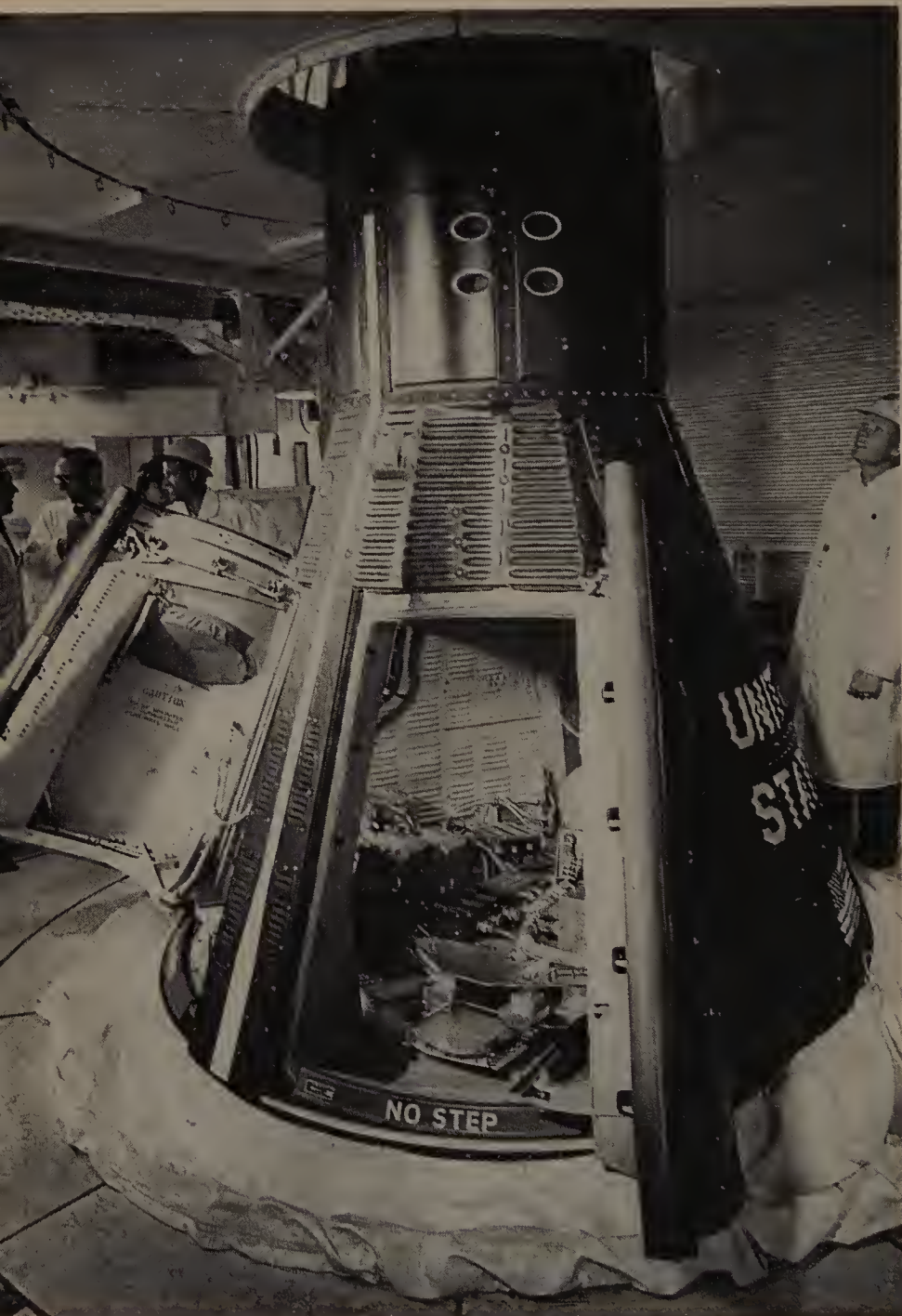
PLATE XLVI A Gemini CAPSULE FOR TWO-MAN SPACE-FLIGHTS. (p. 286)
