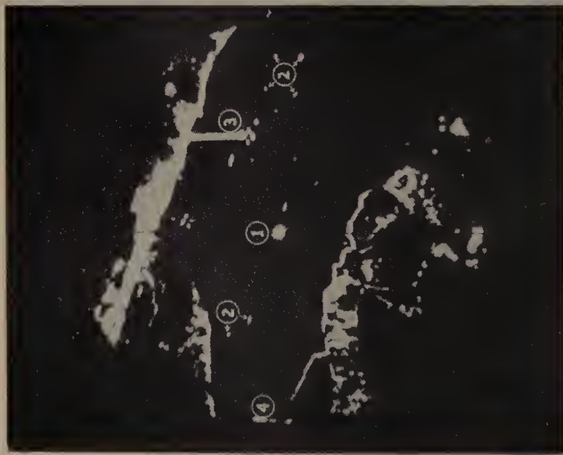
PLATE XXVII RADAR AT THE END OF THE WAR. (Left) The Thames Estuary as displayed on the radar screen aboard ship. The points marked are: (1) the ship that 'took the picture'; (2) other ships and buoys; (3) South-end pier, with ships lying off the end; (4) oiling jetty on south bank of the river. The bright patches round the coasts indicate built-up areas. Compare the map. (Top right) The ship is passing through the boom off South-end. (p. 197)
