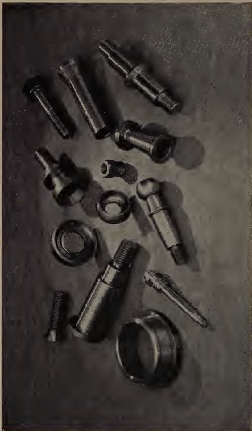
PLATE XXIII SAMPLES OF WORK PRODUCED BY AN AUTOMATIC LATHE. (p. 153)
