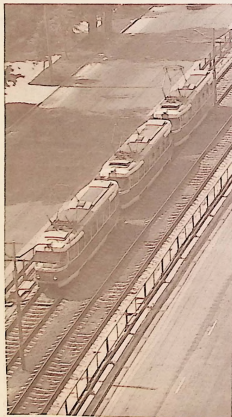
Very high speed "street cars" are proving popular in USSR. Much cheaper to build than subways. All units powered (electric). This is one of several in Kiev.
