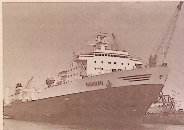
The 'Mukran' is a ferry of a new kind, actually serving as a kind of rail line across the Baltic Sea. One of a fleet being built. These cargo ships are high speed, and carry fully loaded freight trains from Socialist Germany to Soviet port at Klaipeda, and back. Return trip is 48 hours: 40 hours at sea, 4 hours at each dock.
